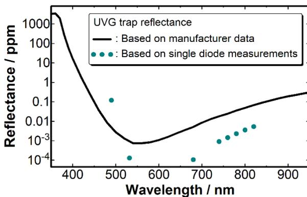
**Figure 3.** Estimated reflectance of the 5-element trap detector based on the single photodiode reflectance provided by the manufacturer (line). The dots show the values based on our measurements on a single photodiode.
