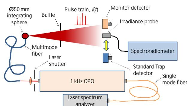
Figure 1. Schematic of the new calibration method
