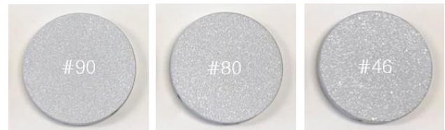
Figure 5. Al plates sprayed with different sizes of Al particles on top of it (#, mesh number)
