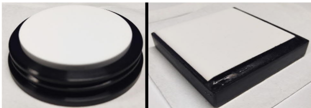
Figure 2. From left to right, a sintered PTFE puck and a matte white ceramic tile
