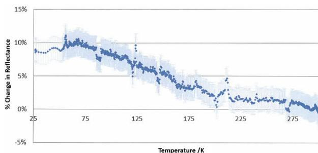
**Figure 2** Preliminary data showing temperature dependence of reflectivity of the VANTA sample. Error bars (95% confidence) account for temperature dependence of setup.
