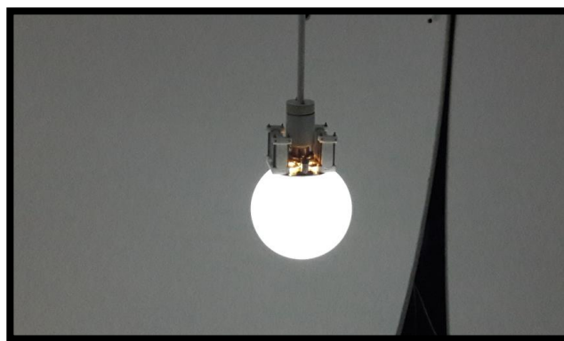
Figure 2. A prototype of a reference lamp with correction filters developed at NSC “Institute of Metrology”
