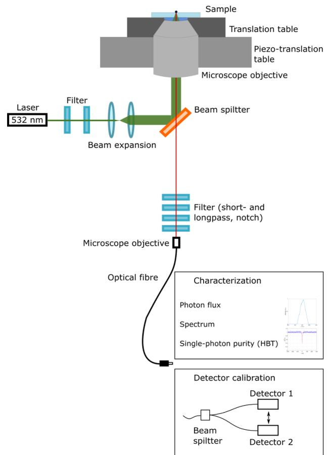
**Figure 1.** Measurement setup used for the characterization and the relative detector calibration.
