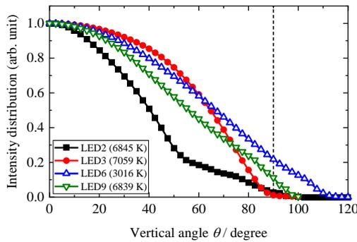
**Figure 2.** Angular intensity distributions of the white LEDs.
