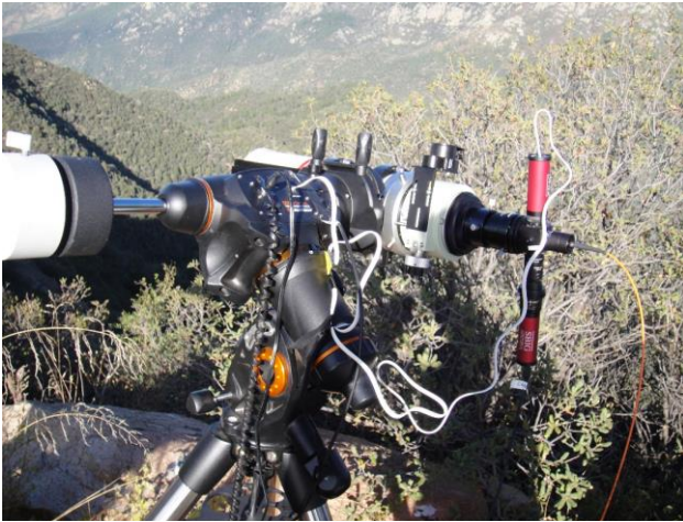
Figure 2 The stellar observation telescope on its mount. On the right side are the red cameras for aligning and guiding on the target star and the orange optical fibre.
