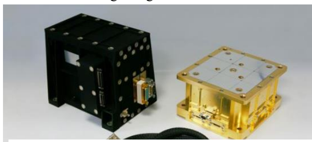
Figure 1. The JTSIM-DARA is composed of a sensor case with 3 radiometer cavities (right) and the control unit.
