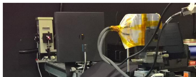
Figure 3. The angular response setup showing the Xe-Lamp in the back, a WG305 filter and a baffle in the middle and the JTSIM-DARA mounted on the goniometer.
